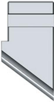
Chamfering Tool Bit
